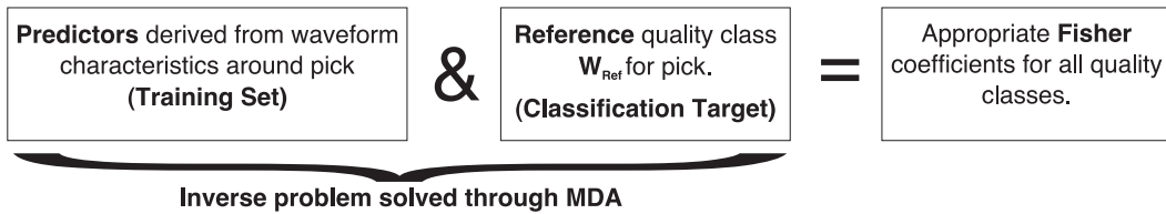
Figure 5: Concept of phase-quality classification with MPX. a) The quality class W_{MPX} of a phase pick is estimated from predictors measured around the pick weighted by Fisher coefficients. b) An appropriate set of Fisher coefficients is derived via MDA from the reference data set (training set).
